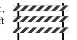
The lines on this barricade angle down to the right, indicating that traffic must pass the barricade on the right side.
