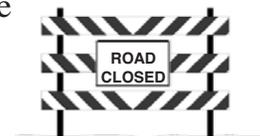
The lines on this barricade angle down to the left, indicating that traffic must pass the barricade on the left side.
