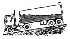
of the liquid. Therefore, forward-and-back surge is very strong. Un-baffled tanks are usually those that transport food products (milk, for example). Sanitation regulations forbid the use of baffles because of the difficulty in cleaning the inside of the tank. Be extremely cautious (slow and careful) in driving smooth bore tanks, especially when starting and stopping.
