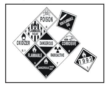
Figure 9-3). Placards must be readable from all four directions. They are 10 3/4 inches square, turned upright on a point, in a diamond shape. Cargo tanks and other bulk packaging display the I.D. number of their contents on placards or orange panels.
