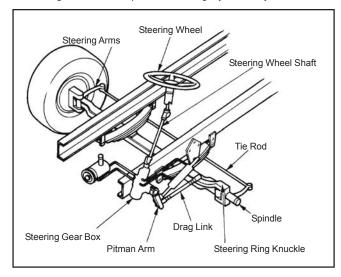
Figure 2-2 Key Suspension Parts
