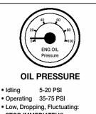
STOP IMMEDIATELY! Without oil the engine can be destroyed rapidly Get In and Start Engine
