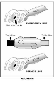
Older trailers do not have spring brakes. If the air supply in the trailer air tank has leaked away there will be no emergency brakes, and the trailer wheels will turn freely. If you crossed the air lines, you could drive away but you wouldn't have trailer brakes. This would be very dangerous. Always test the trailer brakes before driving with the hand valve or by pulling the air supply (tractor protection valve) control. Pull gently against them in a low gear to make sure the brakes work.
