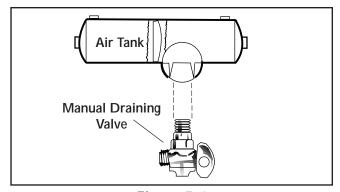
Figure 5-1 Manual Drain Valve
