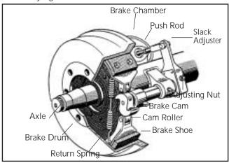
Figure 5-2 S-cam Air Brake
